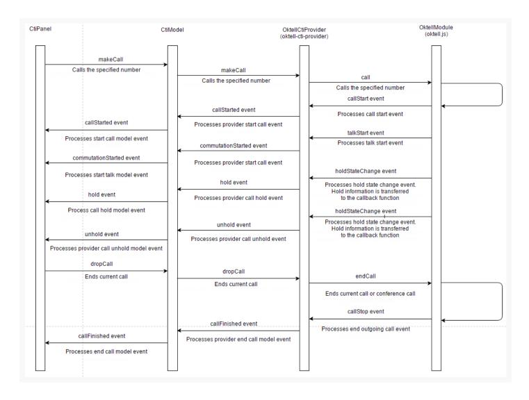
Incoming call of a subscriber 1 to an operator with a consultation call to subscriber 2 with the subsequent connection of the subscriber 1 and subscriber 2 by the operator
