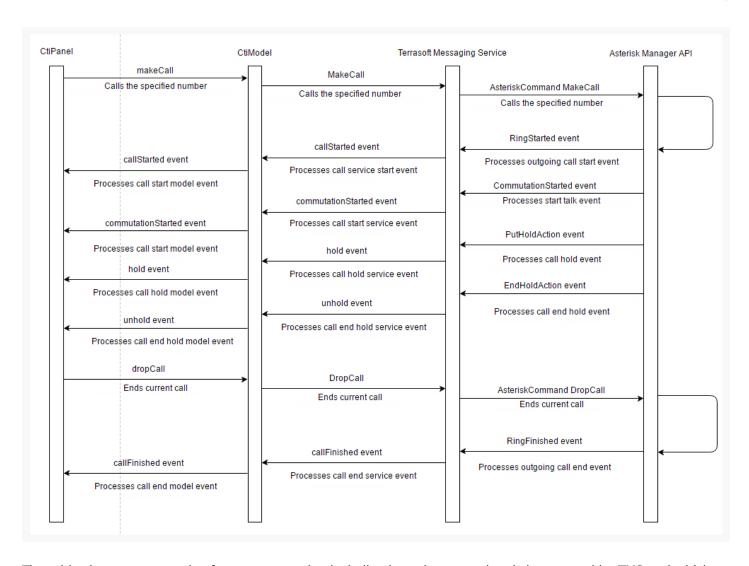
The table shows an example of event processing including how the event data is interpreted by TMS and which values from the listed events are used when processing an incoming call.
